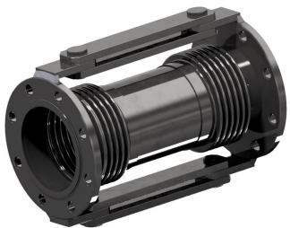
The Expansion Joints ridged hinged mechanism allows them to accept full pressure thrust while being prevented from deflecting axially either in extension or compression. In piping system applications a Double Hinged Expansion joint can be used on its own or in a two or three pin system and can be used in conjunction with Single Hinged Angular Expansion joints as shown.
