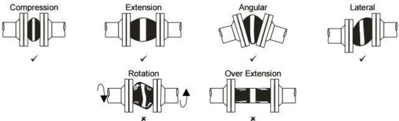
Only the correct mating flanges should be used. They should be the same size and drilling and have a similar sealing face as that of the rubber bellows. They must be clean and free from any debris, sharp edges etc. to prevent damage occurring to the sealing face of the bellows. For mating flanges with a different sealing face diameter a composite gasket should be used to prevent any sharp edges cutting into the rubber sealing face.
