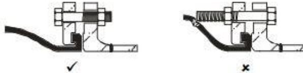
When tied rubber bellows are being used they must be installed at their neutral (supplied) length. Recheck installation length and movement capabilities of the bellows being installed. Ensure that the steel washers and the rubber top hat washers have been correctly fitted. Tie bar assemblies should be uniformly tightened and bolts rechecked after approximately seven days.
