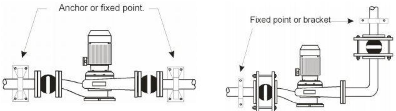
Rubber bellows will exert a pressure thrust in service and must be anchored to protect adjacent pipework and equipment. Rubber bellows will extend under pressure and must be anchored to prevent this happening.
